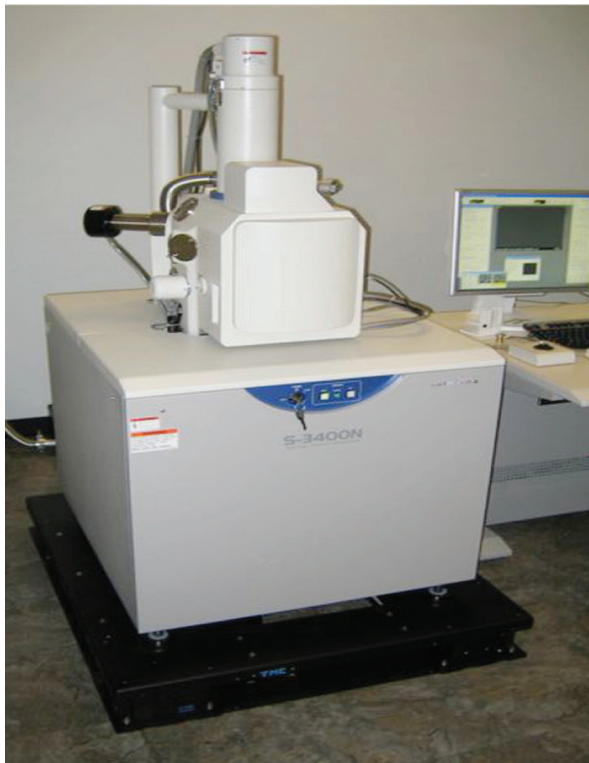
STACIS® iX SEM-Base™ Floor Platform isolating an FEI Helios NanoLab DualBeam SEM/FIB (top left), a JEOL JSM-6700F Field Emission Scanning Electron Microscope (top right), an Hitachi S-3400N SEM (bottom left), and a SEM with EDAX TEXS WDS Spectrometer and EDAX Hikari EBSD Camera (bottom right).
